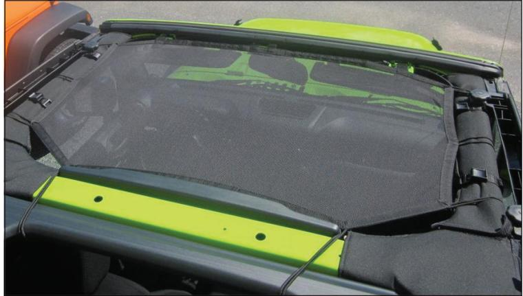
1. Before installing flip soft top to Sunrider feature or lower top to full down position. Freedom panels will need to be removed for installation on hard top vehicles. Slide front side Velcro straps through windshield footman loops and secure (fig.1). Loop rear Bungee straps over factory sports bar and back to strap button (fig.2)
